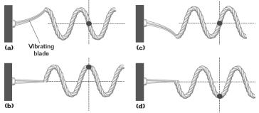
As the sine wave created by this vibrating blade travels to the right, a single point on the string vibrates up and down with simple harmonic motion.
