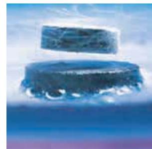
The strong magnetic field produced by these superconducting electromagnets can suspend this 8 cm disk.
