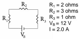
Find Voltage drop at each resistor
