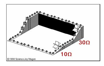
Below is an animation of a series circuit where electrical energy is shown as gravitational potential energy (GPE). The greater the change in height, the more energy is used or the more work is done.
