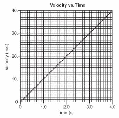
What is the magnitude of the displacement of the car from t = 2.0 seconds to t = 4.0 seconds?
