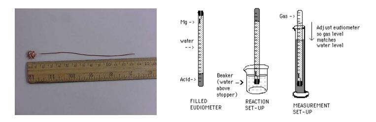
4) Fill the gas measuring tube with 10 mL of acid
