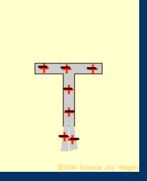
Charged object **does not touch** the electroscope.
