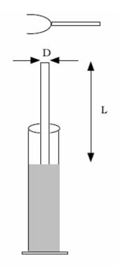
Changing the air length (height) of the tube with a tuning fork sounding above it will result in the column of air vibrating at the same frequency as the tuning fork when the air column length is a harmonic length of the frequency.
