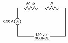
a. Calculate the equivalent resistance of the circuit shown. [Show all work, including the equation and substitution with units.]
